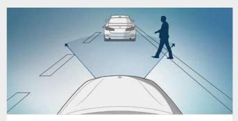
☐ Person warning with city braking function actively assists the driver with the prevention of collisions involving pedestrians. It is active at speeds of up to 35mph and preconditions the brakes for increased responsiveness. In the event of an emergency, the system prevents a collision or ensures that the collision speed is considerably reduced.<sup>2,3</sup>
