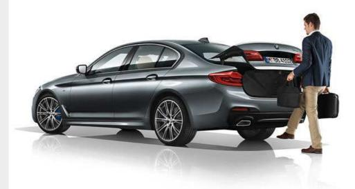
☐ Automatic tailgate operation allows the convenient opening and closing of the tailgate by simply pressing the conveniently located button in the door panelling or on the car key. The tailgate can also be opened in the conventional manner, using the outside handle, and closed using a button on the inside of the tailgate.
