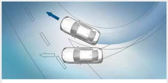
■ Hill-start Assistant constantly assesses the vehicle's movements and stabilises by using engine and braking management when unstable driving conditions are detected. Additional features of Hill-start Assistant are, for example, brake drying, braking readiness or the Hill-start Assistant, which holds the vehicle briefly in place when starting on inclines to prevent it from rolling backwards.
