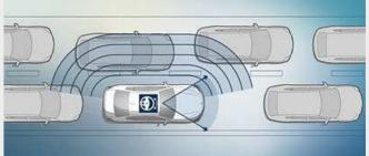
☐ The Lane Departure Warning detects lane markings and alerts the driver before an unintentional lane change at speeds above around 45mph by means of vibrations in the steering wheel. The warning is not activated if the lane change is deliberate, that is, when the indicator has been activated.3
