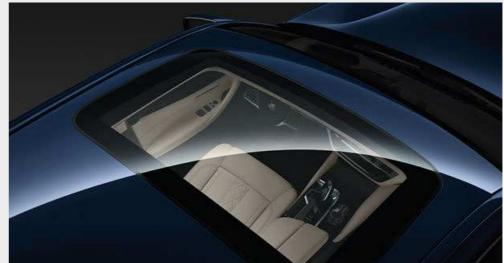
$\hfill\square$  The electric glass sunroof with slide and lift function, including an electric sliding interior roof, anti-trap protection, as well as comfort opening and closing, allows the airflow to be individually regulated to create a pleasant interior climate. The integrated wind deflector prevents draughts from developing in the interior and ensures a lower level of wind noise.
