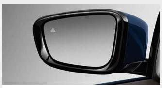
☐ If the indicator is on, the radar-based Lane Change Warning² warns the driver of approaching vehicles in the blind spot as well as vehicles in the neighbouring lane. The system functions beginning at speeds of 6mph, and in dangerous situations, it causes the steering wheel to vibrate and the triangle symbol in the exterior mirror to blink.
