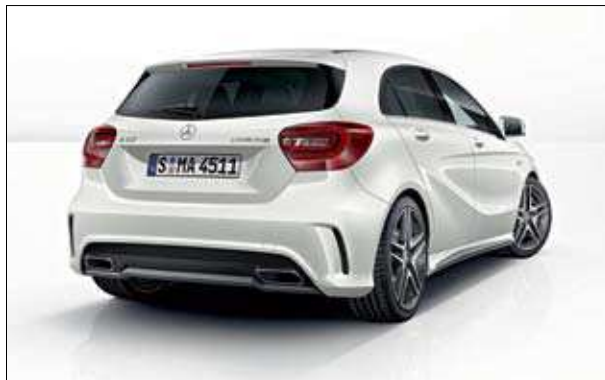
The two-pipe AMG sports exhaust system and AMG-design rear apron.
