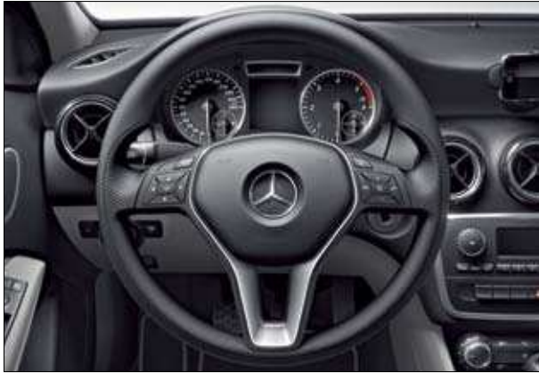
3-spoke multifunction steering wheel with 12 function buttons.
