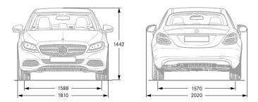
All dimensions in millimetres. The dimensions shown are mean values and apply to standard-specification, unladen vehicles.
