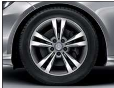
5-twin-spoke light-alloy wheels with 245/45 R 17 tyres (standard for AVANTGARDE for 4- and 6-cylinder models, Code 44R/R38?).
