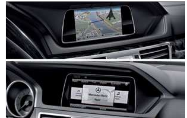
SPLITVIEW displays two different images at the same time – for the driver and front passenger – on a single screen.
