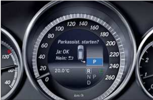
The display in the instrument cluster gives a clear picture of the parking manoeuvres at all times.
