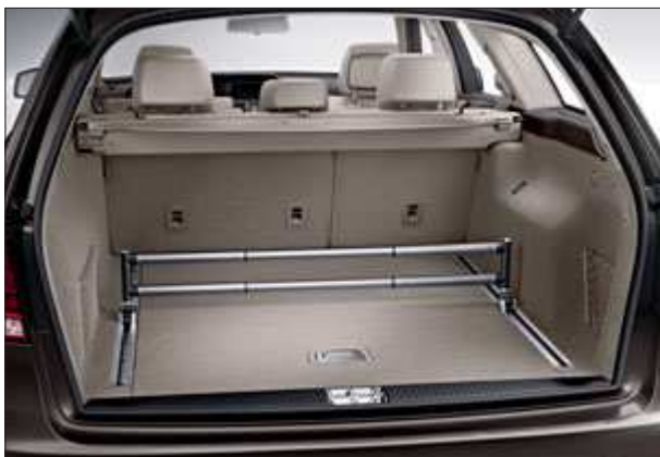
EASY-PACK load compartment management load-securing kit (for estate only).
