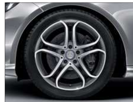
5-twin-spoke light-alloy wheels with 245/40 R 18 tyres at the front and 265/35 R 18 at the rear, in the case of 4MATIC 245/40 R 18 all round (part of the Exterior Sports package, Code 22R/66R).
