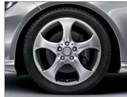
5-spoke light-alloy wheels with 245/40 R 18 tyres at the front and 265/35 R 18 tyres at the rear (option, Code R08/52R).
