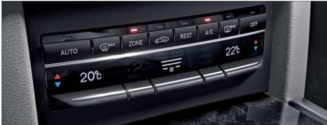
The controls for the THERMOTRONIC luxury automatic climate control system are ergonomic and intuitive.
