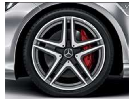
5-twin-spoke AMG forged wheels with 255/35 R 19 tyres at the front and 285/30 R 19 tyres at the rear, painted titanium grey with high-sheen finish (option for AMG models, Code 785).
