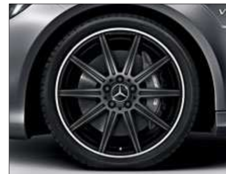
10-spoke AMG light-alloy wheels with 255/35 R 19 tyres at the front and 285/30 R 19 tyres at the rear, painted matt black, rim flange with high-sheen finish (option for AMG models, Code 752).
