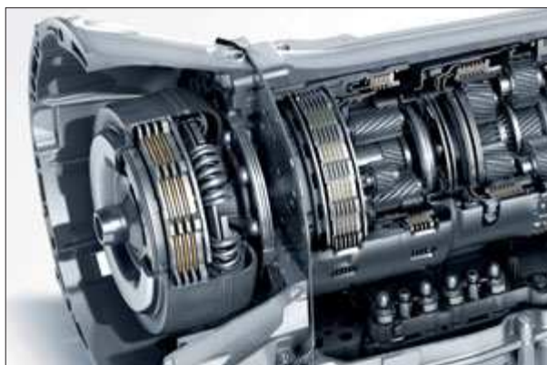
The AMG SPEEDSHIFT MCT 7-speed sports transmission.
